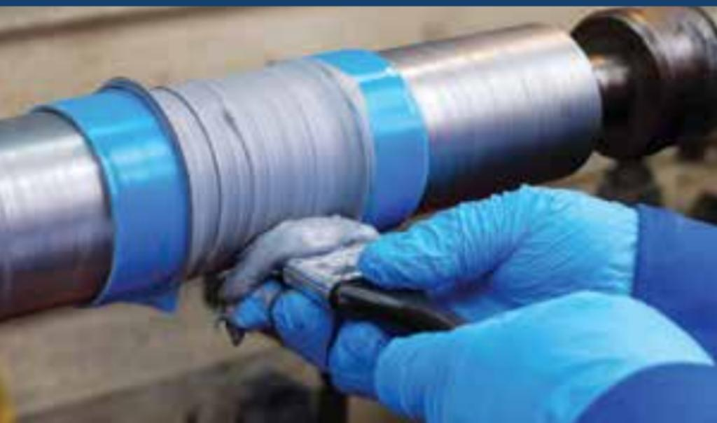
High-performance, paste-grade, and machinable polymers for the repair and protection of metallic and non-metallic components of industrial equipment.
