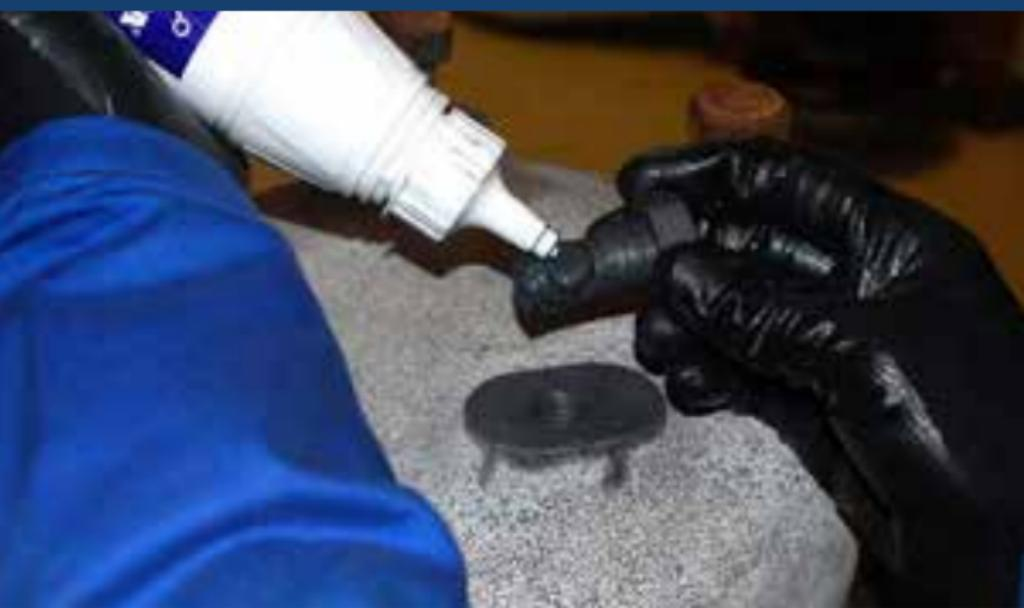
Multi-purpose and high-performance material for preventing seizure and galling of mating components.
